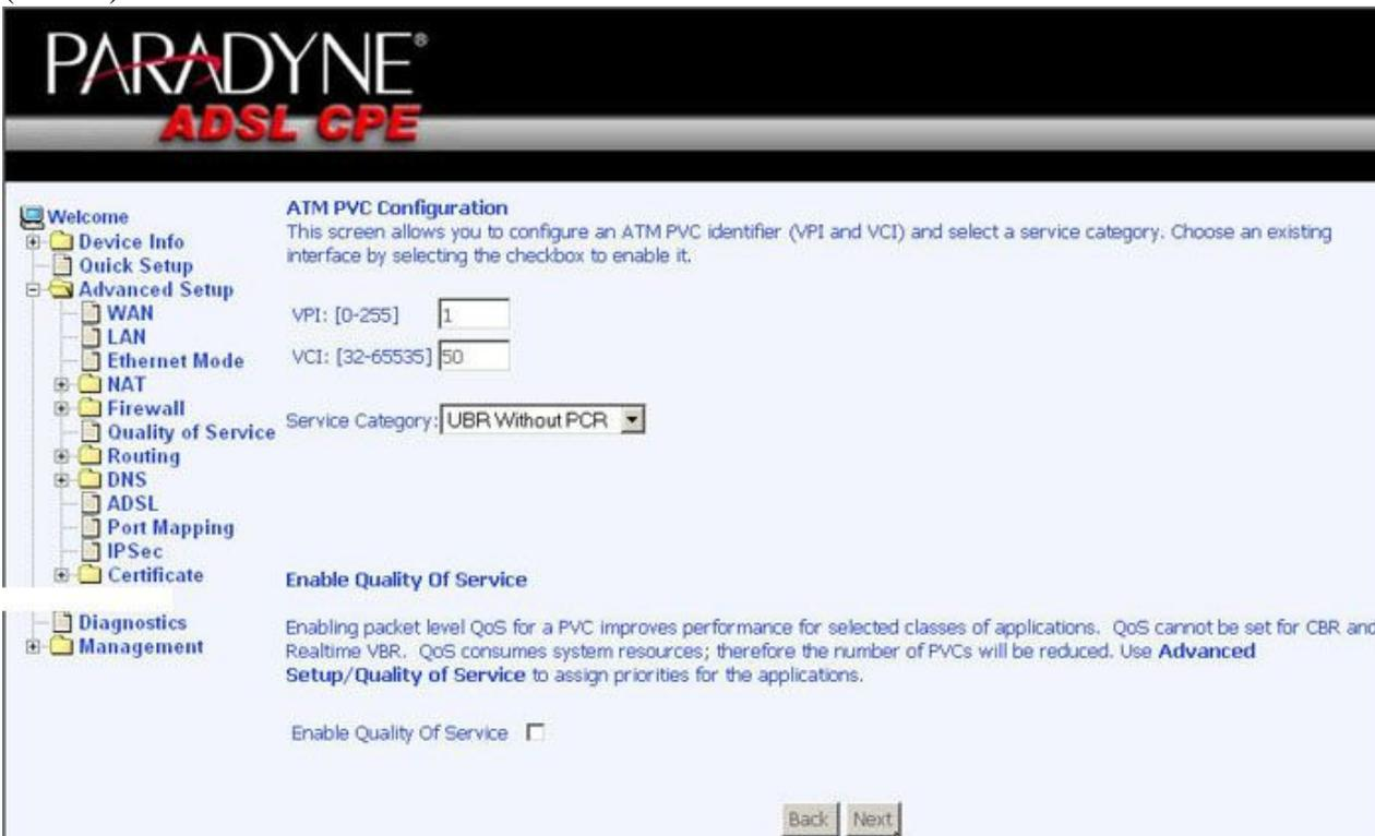
The screenshot shows the ATM PVC Configuration page in the PARADYNE ADSL CPE web interface. The left sidebar shows 'Advanced Setup' expanded to 'WAN'. The main content area is titled 'ATM PVC Configuration' and includes instructions: 'This screen allows you to configure an ATM PVC identifier (VPI and VCI) and select a service category. Choose an existing interface by selecting the checkbox to enable it.' Below this are input fields for VPI and VCI, and a dropdown menu for Service Category.
